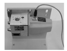
1. Fix the unit without cartridge in vertical mounting position. If possible, place a drip tray or similar under the unit to prevent environmental pollution.
