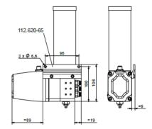
When using oil as the delivery medium, an installation position in which the cartridge stands vertically is preferred in order to ensure air-free delivery of the medium.
