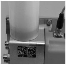
For better ventilation when using oil, the unit should be actuated during the entire filling process and fixed with the outlets inclined upwards.
