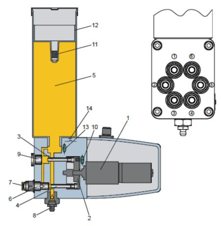
The rotational movement of an electric motor 1 is converted via a swash plate 2 into a lifting movement of the delivery pistons 3 and 4. In the suction position (piston 4) the medium is drawn in from the cartridge 5, in the pressure position (piston 3) the medium is pumped towards the outlet.
